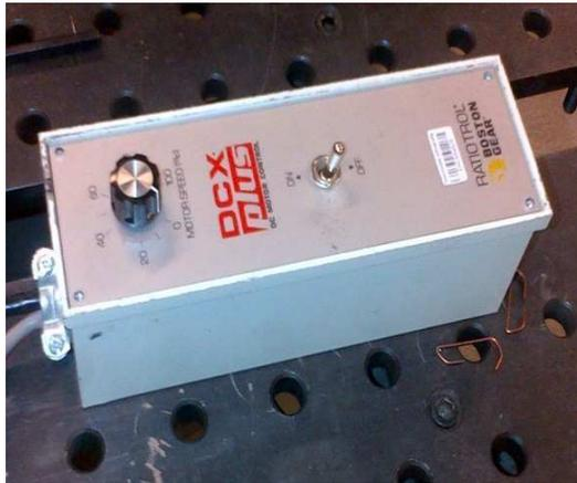
**Figure 34 : Motor Speed Controller**
