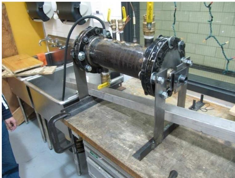
**Figure 57: Liquid Leak Test**
