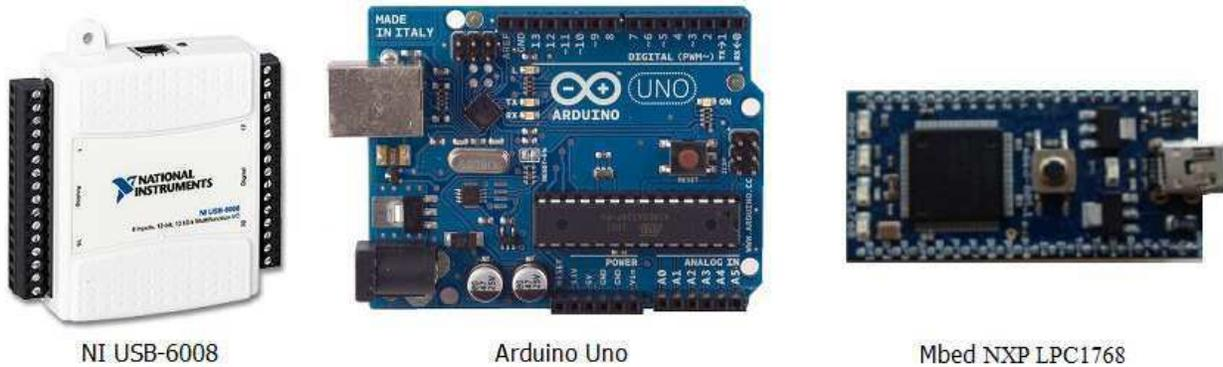
**Figure 18: DAQ Boards & Microcontrollers**
