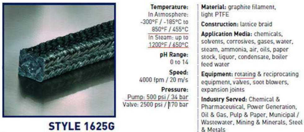
Figure 32: Packing Seal Specifications [14]
