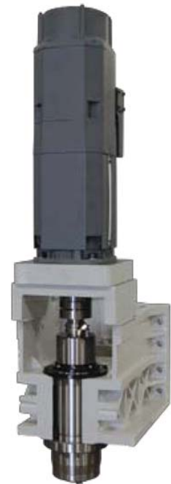
Pictured above: Inline spindle with inline coupling and 35 HP spindle motor. The casting is cutaway to illustrate the coolant cavity surrounding the spindle cartridge.
