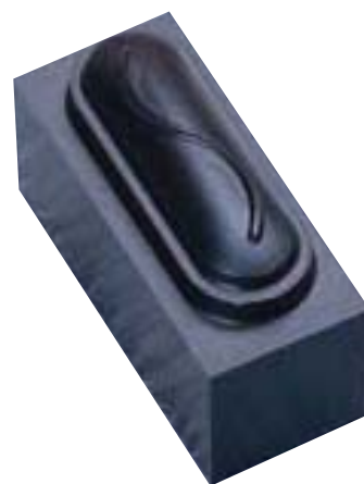
Part machined on a Milltronics CNC control with Feed Forward error correction
