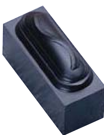
Part machined on conventional CNC control without Feed Forward error correction
