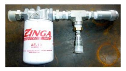
b) The parts for this are (from left to right): 1" nipple, Oil filter and header, 1" to 3/4" reducer, 3/4" nipple, 3/4" T adapter, 3/4" to 3/8" recucer, 1/4" quick connect, 3/4" T adapter and 3/4" quick connect.
