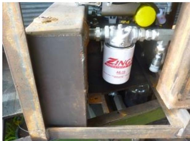
8. Connect the 1" suction hose between the strainer and the pump intake.
