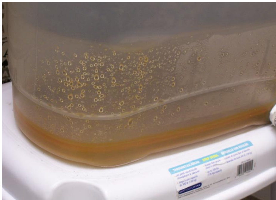
Bioleachate Sample (day 13 Iron deposits)
