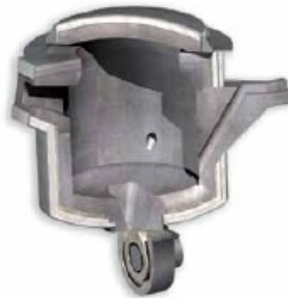
Holding channel furnaces
