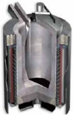
Coreless induction furnace
