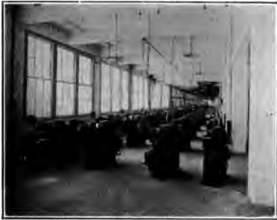
From ribbon to completed tube in one operation. Each machine makes 20,000 tubes a day.
