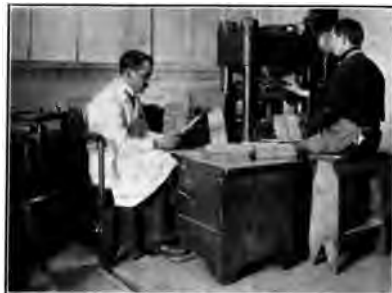
Hydraulic pressure of 40 tons secures the positive tubes in a steel grid, the last operation in the construction of a strong, durable positive plate.
