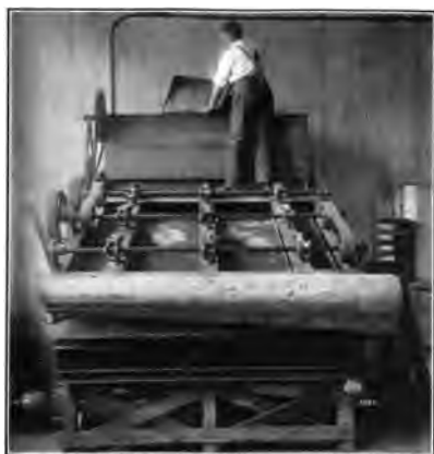
After drying over steam coils the flake is carefully screened
