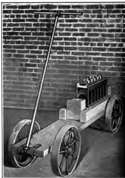
When Fig. 2 test was completed, the Edison Battery was mounted on this truck and the truck projected against a brick abutment 1,000 times at speed of 15 miles per hour at moment of impact before Mr. Edison would "pass" it.
