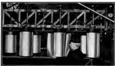
Stripping copper-nickel sheet from cylinder. The sheet is .0075 inch thick.
