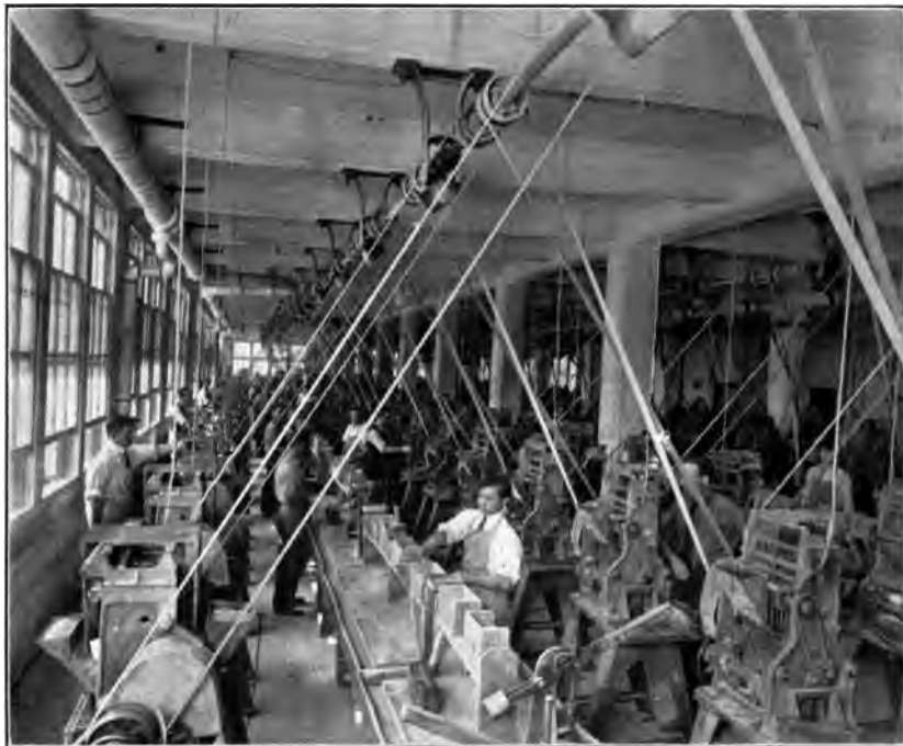
Loading 630 layers, alternately nickel hydrate and nickel flake, into a tube \frac{1}{2} inches long. See magnified section of tube above.
