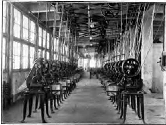
The negative pocket "halves" are formed from the ribbon by one blow in these perfected die-stamping presses.
