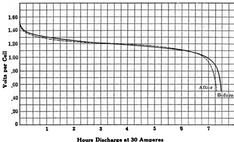
Fig. 3—Effect of Shock Test (A4 Cell). Normal rate discharges before and after the 13.5 lb. cell was lifted and dropped one-half inch on solid wood 1,776,000 times. Cell had normal rate overcharge in each case.
