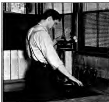
Making the Edison Container a one piece can by oxy-acetylene welding.
