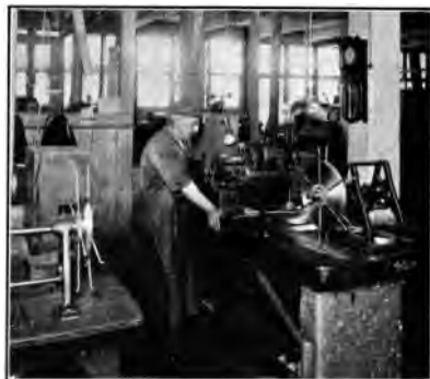
Perforating carbon steel ribbon, 560 holes to the square inch.
