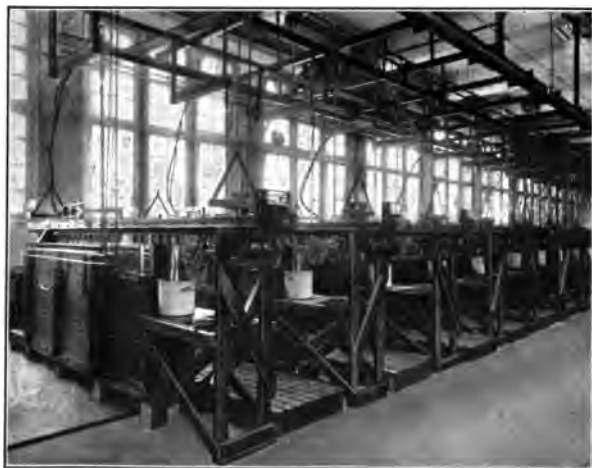
Traveling in and out through a series of baths, the perforated steel ribbon is subjected to a continuous nickel-plating process.
