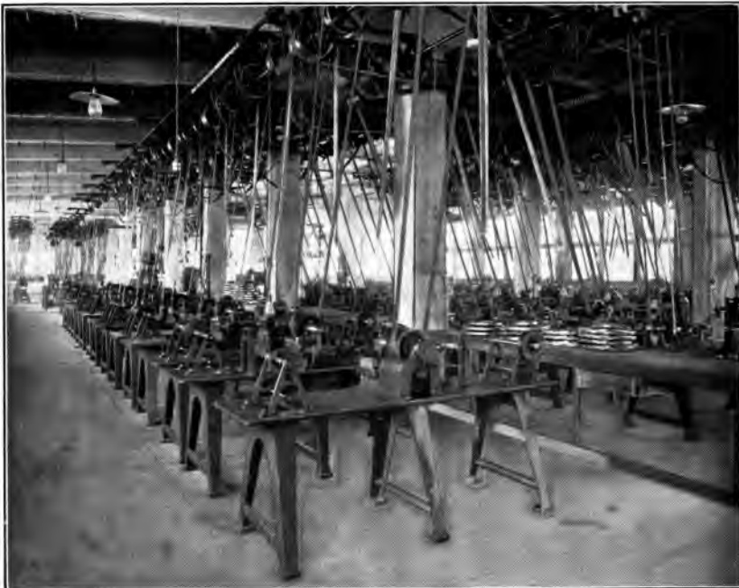
Perforating machinery. The active material is held in tubes and pockets made of perforated steel ribbon. The cutting and finishing of these perforations is one of the most interesting processes in the manufacture of the Edison Cell.
