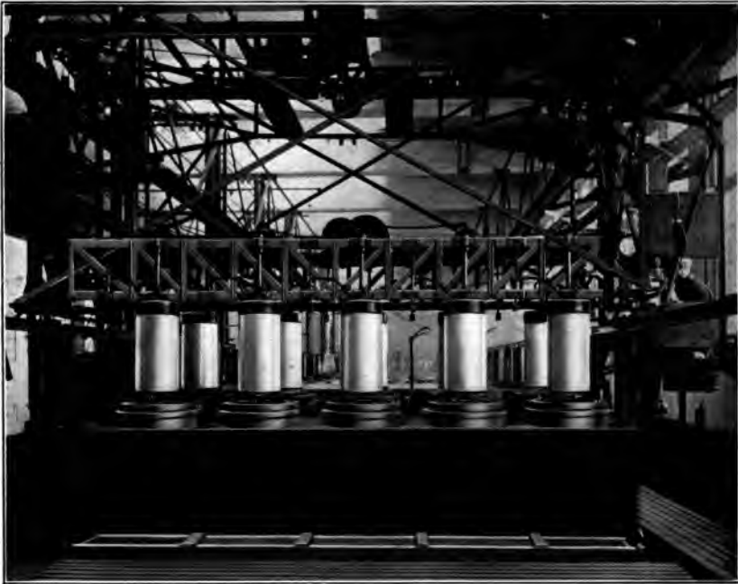
The first process in making nickel "Snow Flake." Plating 250 alternate layers of extremely thin nickel and copper on revolving cylinders.
