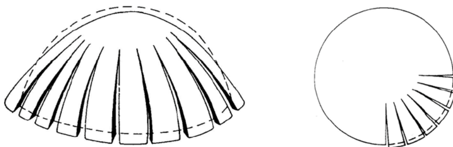
Fig. 94 – Settling behaviour of domes (Heyman 1995)
