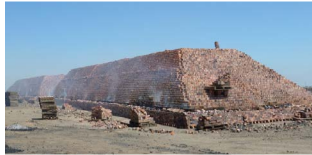
Figure 2: Operation of a Clamp Kiln in South Africa
