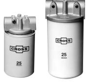
The CROSS SF series hydraulic filters feature spin-on, throw away type cartridges. SGF models also include the condition indicator. These units provice full flow efficiency up to the cracking pressure of the through-type bypass relief valve. Good filtration with regular element changes is essential to protect hydraulic components from damage due to contamination. Please see HYDRAULIC SAFETY SHEET (Page 18).
