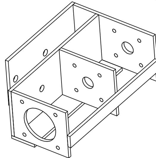
Fabricated Mounting Frame from 7 Pieces 1/2" Steel Plate
