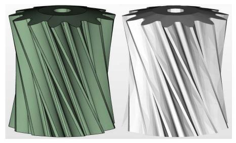
The main difference between mechanical CAD products and the 3D tools used in other industries is that mechanical designs need to be extremely precise. Modern CAD tools can represent holes a micron in diameter on parts that are a kilometer long. These models are commonly called "precise solids," or more technically, "boundary representation" (B-rep) solid models.
