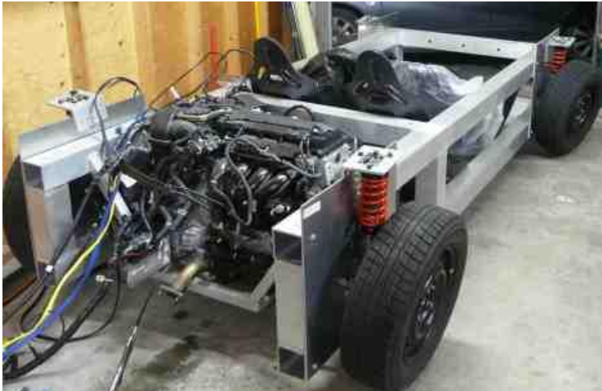
WIKISPEED Fig. 1 TD2-1-1a Power train components (Honda R18A).
