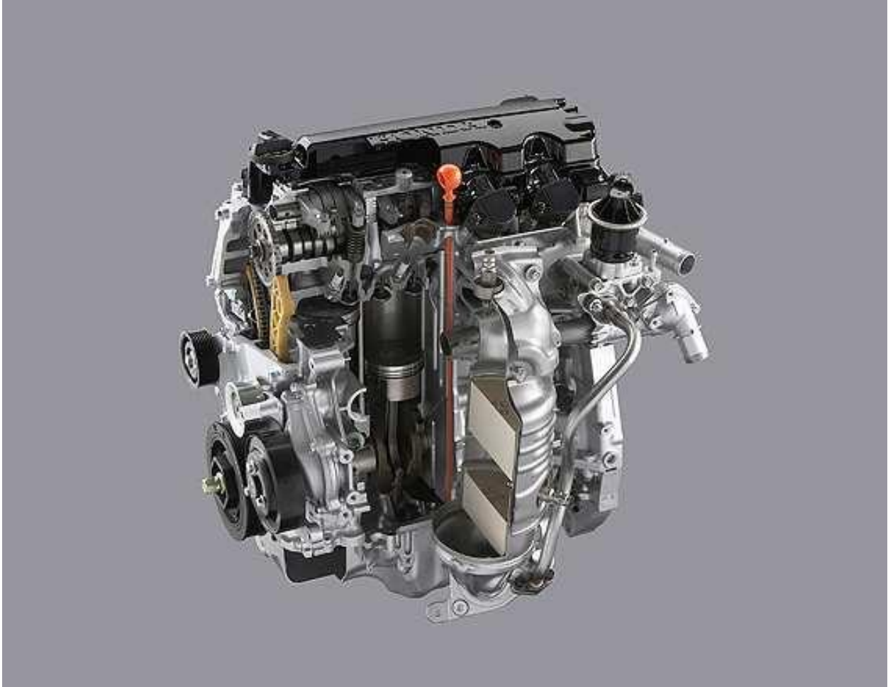
WIKISPEED Fig. 3 TD2-1-1c Exhaust header integrated catalytic converter, shown attached to R18A engine, cutaway view. Note double block elements and immediate access to hottest gas for rapid element heating and exceptional cold start emissions control.
