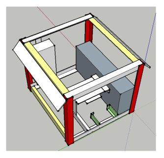
c) After the mount has cooled, lower the battery into the rectangle to verify a proper fit.
