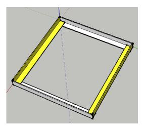
b) With one welded rectangle on the bottom, position the 24" pieces outside corner joints as shown below. Check that the angles are square, then tack and weld securely.
