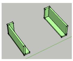
b) Weld the two mounts to the angle iron and tank to form a rectangle for the battery as shown below.
