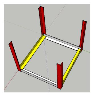
c) Position the second rectangle as shown below, then tack and weld. Inspect all corners to verify secure welds.
