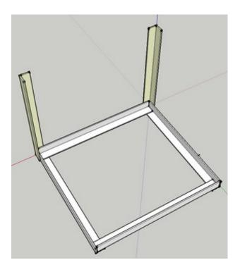
c) Position the second rectangle as shown below, then tack and weld. Inspect all corners to verify secure welds.
