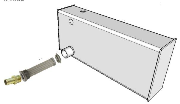
b) Secure the hydraulic tank to the frame with clamps, then weld it with 4 x 1" welds. The tank is ¼" and it can be easily damaged by over-heating. Spacers may be needed on the sides near the top to keep everything snug.
