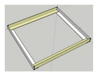
b) With one welded rectangle on the bottom, position two 24" pieces outside corner joints as shown below. Check that the angles are square, then tack and weld. Note: The optional jig makes this much easier and accurate. Repeat the prior procedure and this one for another half of the frame assembly.
