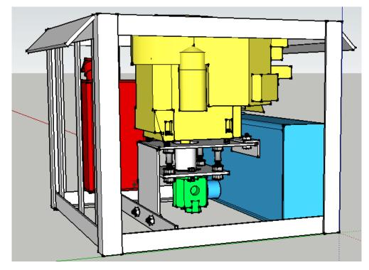
i) Thread the ½" x 2" engine mounting bolts each about half-way with nuts, then lift each side of the motor and insert the bolts into the engine mounting holes. Adjust the nuts so the space between the plate and the engine is ½" and the engine rests evenly on all four bolts. Lightly weld the bolts in place to the plate.
