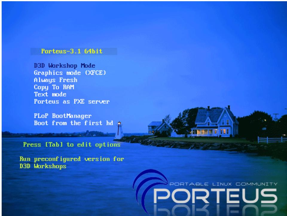
Figure 3: The screen that the tested D3D-Porteus boots into. Pressing Enter loads D3D-Porteus into RAM and starts Pronterface in full-screen mode. This screenshot was taken by booting the D3D-Porteus ISO on a virtual machine created by the program VirtualBox.
