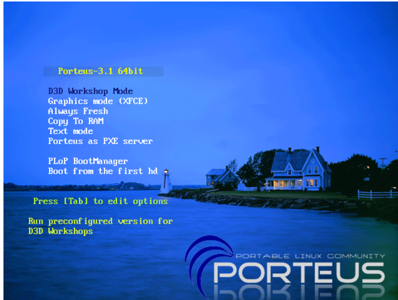
Figure 2.1: The screen that the tested D3D-Porteus boots into. Pressing Enter loads D3D-Porteus into RAM and starts Pronterface in full-screen mode. This screenshot was taken by booting the D3D-Porteus ISO on a virtual machine created by the program Virtual-Box.
