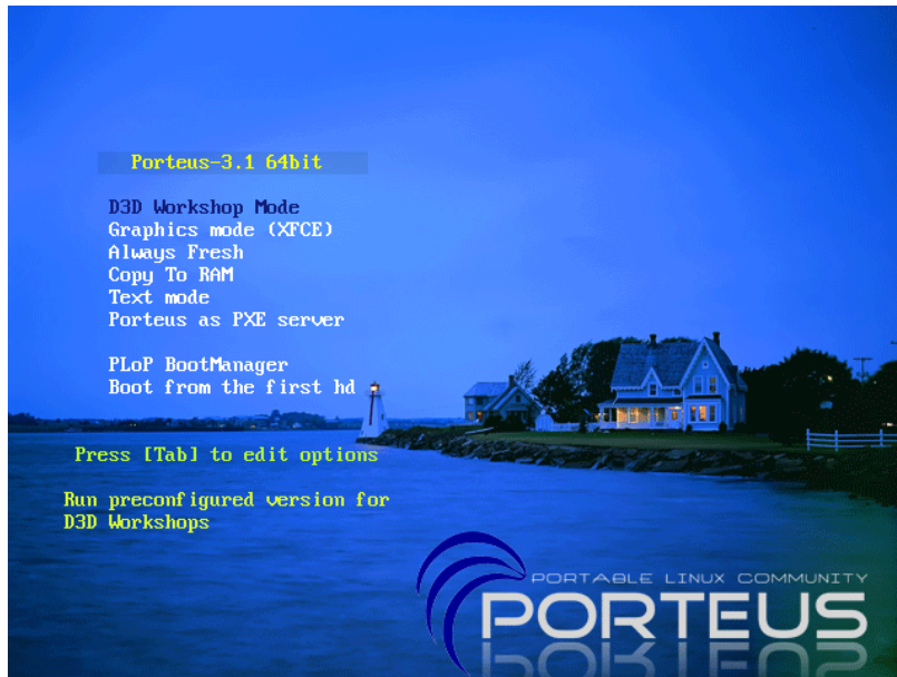
Figure 2.1: The screen that the tested D3D-Porteus boots into. Pressing Enter loads D3D-Porteus into RAM and starts Pronteerface in full-screen mode. This screenshot was taken by booting the D3D-Porteus ISO on a virtual machine created by the program Virtual-Box.
