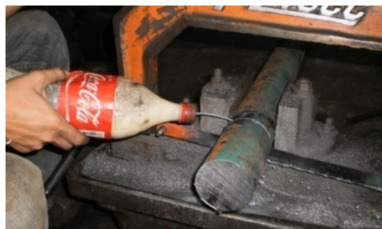
Figure 9. Cutting thick cross sectional steels can be efficiently cut with the use of Coco Cutting Fluid manually.
