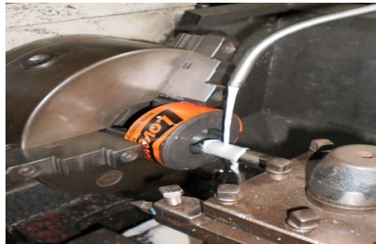
Figure 9. Cutting thick cross sectional steels can be efficiently cut with the use of Coco Cutting Fluid manually.
