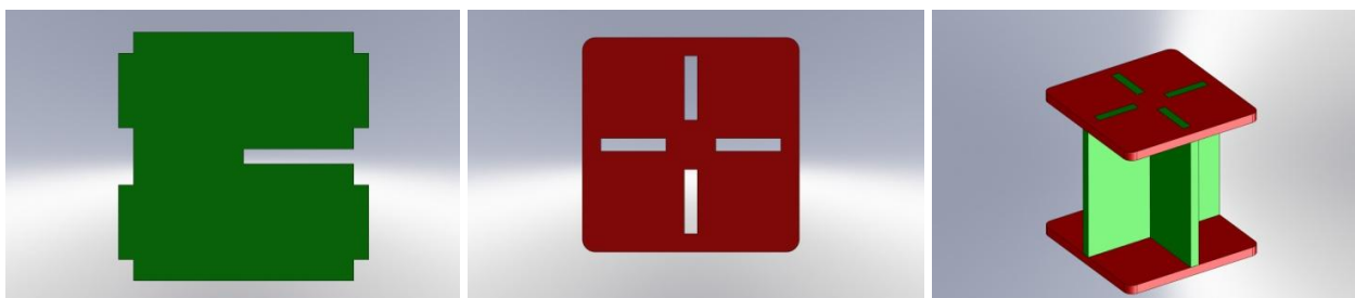
Figure 4. nLMD example with 4 plates (2 in X, 1 in Y, 1 in Z).
