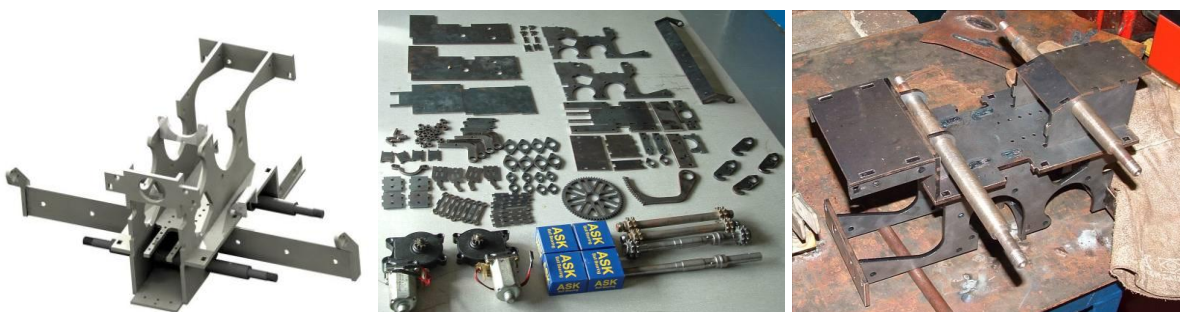
Figure 10. Design, Manufacture and Assembly of the ultrasound Robot.
