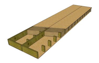
can be toe-nailed through end blocks edge nailed along OSB
