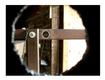
Now insert the 2" x 2 3/8" round tube into the hole in the Cant rail. Insert the loader arm pivot bar
