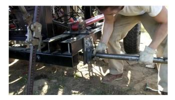
Before passing the axle shaft through the inner bearing, slide on a large washer and two locking collars.
