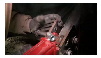
Mount the hydraulic cylinder frame plates to the frame.
