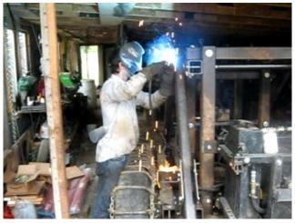
Remove the loader arms and completely weld the loader arm round inserts, then grind them smooth.
