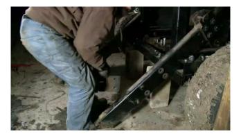
Position the hydraulic cylinder between the loader arm cylinder plates and secure with a pin and cotter pin (2 total).
