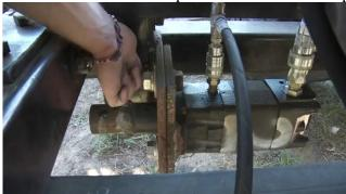
Attach the bearing to the axle shaft mounting plate so that the bearing is facing outwards. Bolt the plate to the frame with 3/4" x 5 1/2" bolts (8 total).
