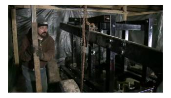
Slide lock collars onto the shaft outside of the loader arm but don't tighten them all the way. Bolt the
