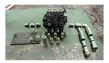
First, you must cut off the end of the power beyond sleeve to prevent it interfering with the return flow. If available, place the part into a band saw. Otherwise just use a vice, a hacksaw, and a steady hand. Either way cut off the tip just below the threads.
