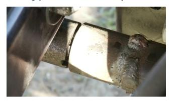
Now the hydraulic motor, axle shaft, and axle bearings are all lined up properly. Weld the motor mount plate to the C-pillar. Seriously, weld it on there nice and tight. All the way around. Also, tack weld the bearing mount plates to the horizontal tubes. But just tack weld those so it's easy to grind the weld off later if necessary.
