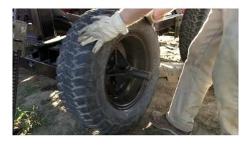
Secure with a 3/4" x 4 1/2" bolt and lock nut (4 times).
