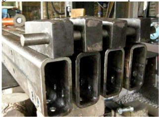
Weld all the way around the insert to finish attaching it to the loader arm. Grind the welds smooth.
