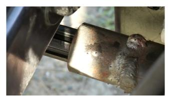
There should be no more than 1/8" gap between the female coupler and the shaft face.
