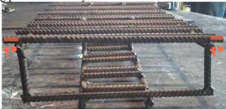
Make the bottom of the welding jig by first laying out the remaining two long pieces of rebar (part WTWJ#1) 5 inches apart (on centers). Lay 24 pieces of rebar (part WTWJ#3) along the length of part WTWJ#1, using the same spacing as the top part of the jig. Do not let part WTWJ#3 overhang WTWJ#1 at all.
