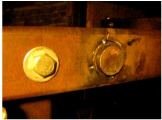
Mount the loader arms on the loader arm pivot bar, with the 2 3/8" insert in place.
