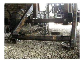
Tack weld the outside of the loader arm 2 3/8" round inserts so they are in proper alignment with the loader arm pivot bar and the Cant rail inserts.
