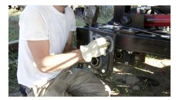
Insert the axle shaft through the outer bearing.
