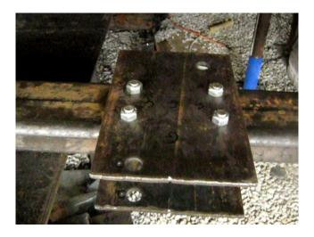
Position the loader arm crossbar mounts (part LACM) on what will now become the inside of the loader arm. Keep in mind the insert is on the bottom of the loader arm. Attach part LACM with two bolts and repeat as necessary.
