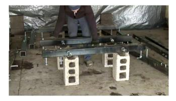
Lay the 4 Base pieces on top of the 3 Sub-Base pieces and line up the bolt holes. Bolt them all together using washers and metal lock nuts. However, do not tighten the bolts. Leave some wiggle room until the entire frame is together.
