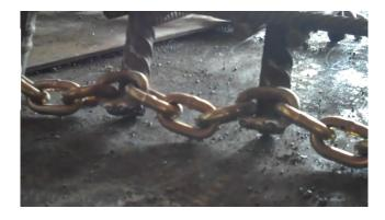
When that's done, flip the jig over and weld the bottom of each link to the TRACK.
