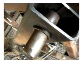
Attach the loader arm crossbar to the supports on both loader arms. Only use one or two bolts because you're going to have to take it apart again.
