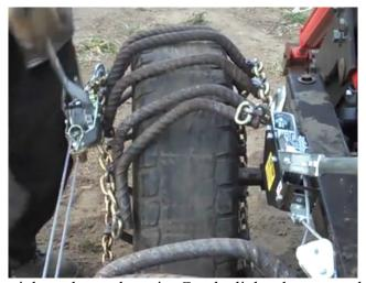
Let air out of the tires, then tighten the track again. Get the links close enough that you can connect them with detachable chain links. Do that, then secure with a cotter pin.
