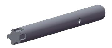
The axle shaft (part AXLE#1) should already have a hole in one end with two slits in it. If not, reference the Cut List.
