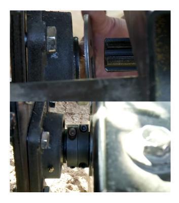
Continue pushing the axle through the inner bearing. Slide on another large washer and lock collar. Continue pushing the shaft until the splined part engages the hydraulic motor unit.
