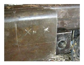
It is best to line up all the loader arms and plugs at this point so that they will have identical pivot points. Run a piece of round bar through the 2 3/8" hole at one end and the inserts (part LAI) at the other. Weld through the plug weld holes so that the insert becomes part of the loader arm.
