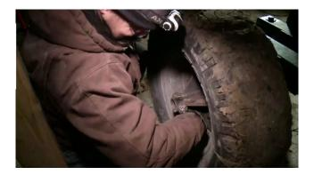
Bolt the wheel mount to the outside of the wheel with 8 bolts and locknuts.
