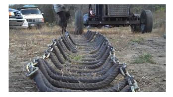
Lay out two complete tracks on the ground the same distance apart as the tractor wheels. Drive the tractor on to the center of the track.
