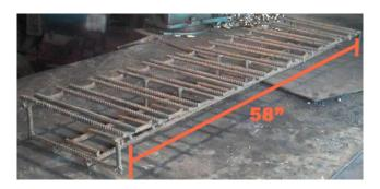
Make the top of the welding jig by first laying out two long pieces of rebar (part WTWJ#1) 13 1/2" apart (on center). Lay twenty four pieces of rebar (part WTWJ#2) across. Position part WTWJ#2 in pairs 1 11/16" from center to center and 3 1/4" apart down the whole length of part WTWJ#1.
