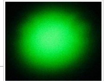
A 5 mW green laser pointer beam profile, showing the TEM 00 profile
