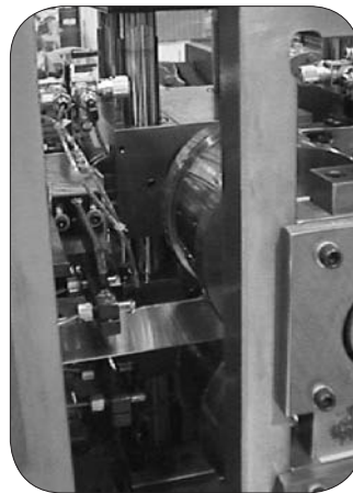
The heat transfer core manufacturing line consists of over 13 stations. Each station has two dies that progressively form the approximately 1/2" wide metal into core components at a rate exceeding 50 fps.
