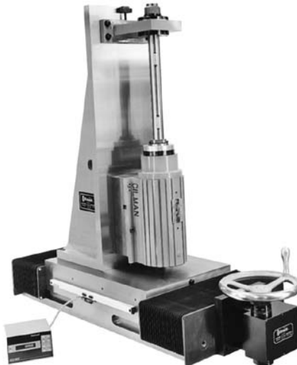
DC20/GMS special compound assembly. Spindle is a 5 H.P. integral motorized assembly with a special arbor and outboard bearing support. Slide is a DC20 with a LRA drive and digital scales. The assembly is used to machine wing sections for the commercial airline industry.
