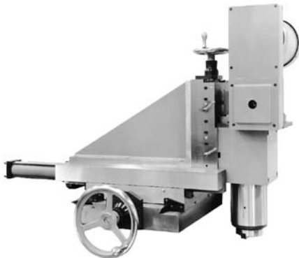
Three-axis dovetail slide and extended 6500 vertical spindle assembly. Two axis manual positioning with hydraulic powered axis motion. Application: machining a horizontal cavity in steel castings.
