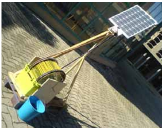
Solar Washer: French Design Students Re-uses bike hubs and bamboo > Solar panels aren't affordable for the average rural African
