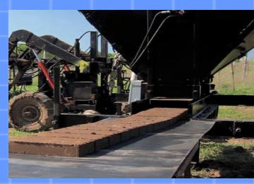
**The Liberator** The world's first open-source compressed earth brick press
