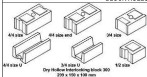
These blocks are used for building disaster-resistant constructions, as they have provisions for vertical and horizontal reinforcing elements. They are dry stacked and a concrete grout is cast in the holes to bind all vertical and horizontal joints.
